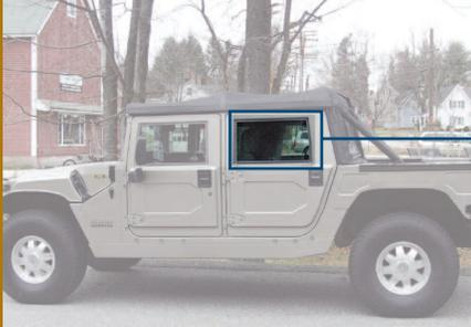
Fractal antenna technology, implemented in transparent conductive film, makes covert capability possible with a mission-capable antenna system that operates over a huge frequency range.
